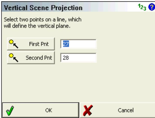
**Note:** You need to measure and store the points that will be used to define the vertical mapping plane, prior to starting the Vertical Projection command.
