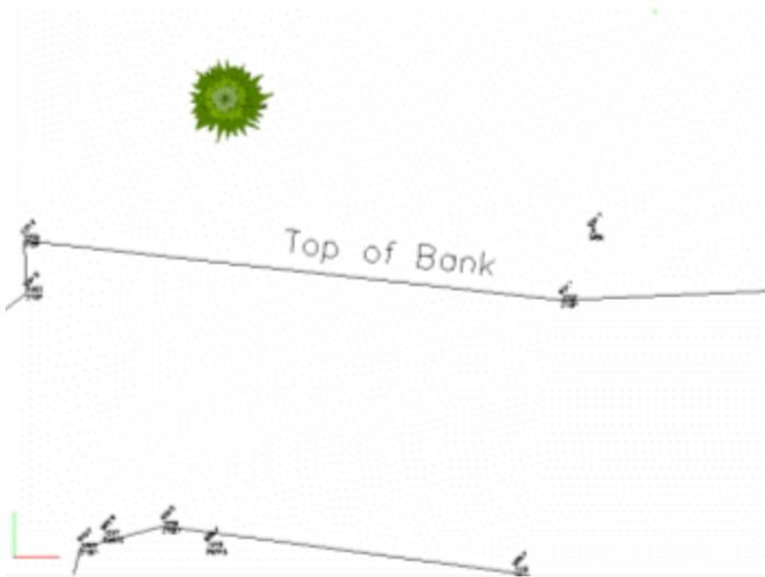
This line represents a location on the site where the slope changes from a steep hill to a relatively flat area.
