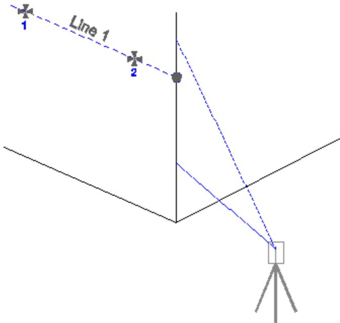
An example of where you might use this is to locate the corner wall of a building. Simply shoot two points on one of the walls, then turn the instrument so it is pointing anywhere along the corner of the building. This command is intended to be used with reflectorless total stations.
