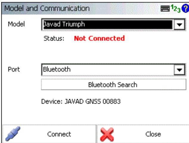
Please note that not all bluetooth-enabled devices will list Bluetooth as a Port option. In some cases you must configure and use a virtual COM port through Windows CE's internal Bluetooth Settings, for example COM6.
