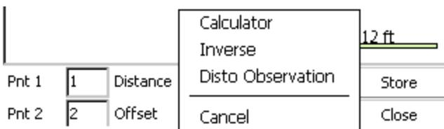
Select "Disto Observation" which will then set Evidence Recorder in a "waiting" mode. Take the measurement with the Disto, press the Bluetooth icon on the Disto, and the measured distance will be accepted by Evidence Recorder and will appear in that distance field.
