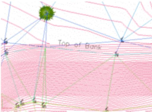
With a breakline, the contours are forced to honor the line, as a change in slope that helps the contours to look correct.
