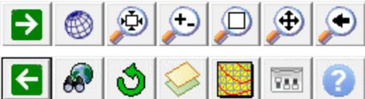
The display toolbar, located at the top of the map screen, is used to zoom, pan, change 3d perspectives, and for displaying information.
