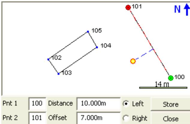
In this example, the baseline is from point 100 to point 101. You will see that an orange dot is displayed in the drawing at the location defined by the point 10m down the baseline and offset 7m to the left.
