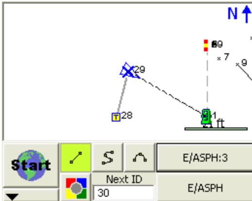
Note the insertion of ":3", this is the group number. Re-use of the Description E/ASPH for a new line series in the current project will automatically increment the group number by one. This allows you track and store multiple active lines of the same description without the need for multiple entries in your AutoMap Library. For example, E/ASPH2, E/ASPH3, E/ASPH4...9 can now be replaced with a single E/ASPH entry.
