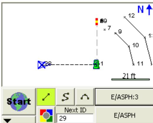
After the second point for this line has been recorded, the first segment will be created. From this point forward, simply continue taking shots to add to the now current Active Line: E/ASPH:3
