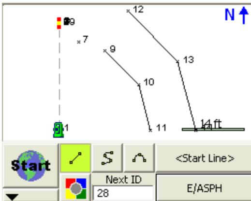
After the shot to the first point for the new line is complete, the line will be added to the Active Lines list, identified by the current point description and an automatically assigned group number: E/ASPH:3. The group number is three, because this is the third figure using the description E/ASPH.
