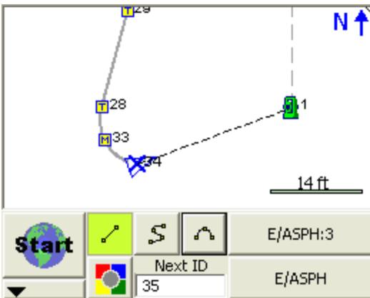
Multiple three point arcs can be connected in series as shown below.
