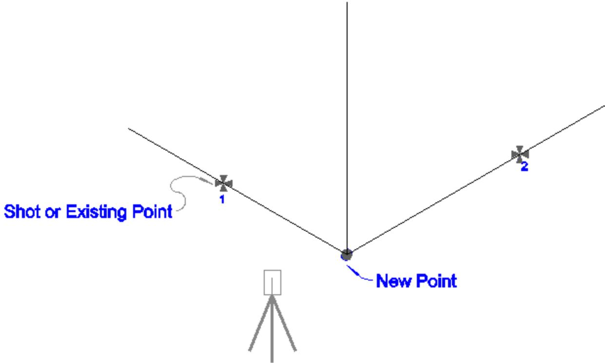
An example of where you could use this is to pick up the corner of a building, whose corner can not be scene from the total station. You could take two shots on one wall to define the reference line, and then take another shot on the intersecting wall. A perpendicular intersection will be computed, which in this case would be the corner of the building.
