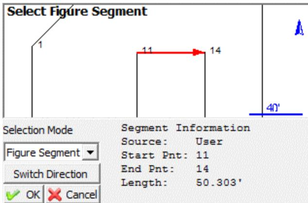
Whichever Selection Mode you use, the selected line will be highlighted in red in the map screen along with a direction indicator. If necessary, you can press the **Switch Direction** button to reverse the start and end of the selected line. Press OK to accept the selected line and proceed to the next step.
