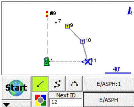
In the example shown, notice E/ASP:1 on the button. This is the current Active Line. E/ASP is the point description and 1 is the group number (added automatically). Since this is the first figure in the map, it is assigned group 1.
