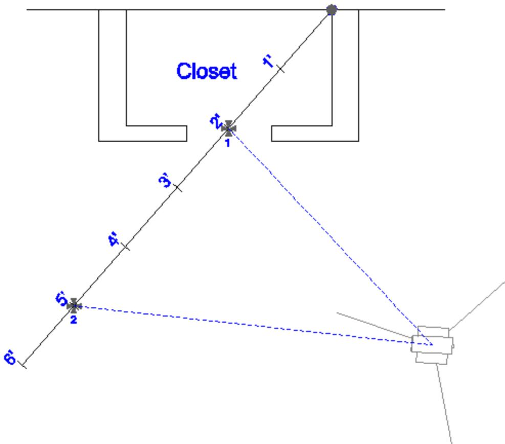
After you take your two measurements, all you need to define is the offset distances. In this example, the corner is two feet to the right of the first measurement (point 1), and 8' up from the floor. After you define the offset directions and offset amounts, you can press the **Store Pnt** button to store the new point.
