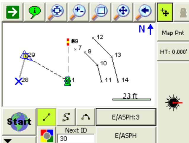
To change the current line, simply select the active line button which will open the Select Figure from List screen. In this example it is the "E/ASPH:3" button.
