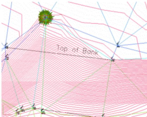
Without a breakline, the contours "flow" over the top of the bank and the contours do not look correct.
