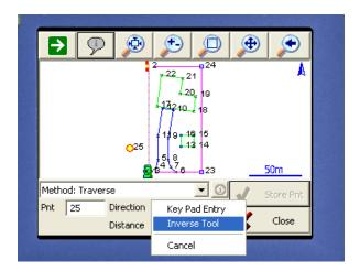
**Info button on Traverse / Intersect Toolbar -** Also added was an info button on the traverse/intersect toolbar. If you press this it will display the results so you can confirm your calculation before storing it.
