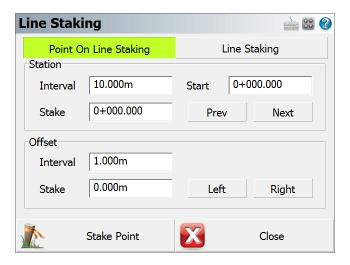
If you want to stake a specific point along the line, select the Point On Line Staking button and specify the station/offset distances then press the **Stake Point** button which will display the <u>stake point</u> toolbar for the specified design point.
