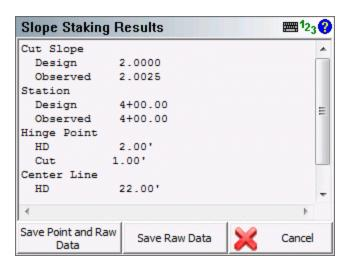
**Cut or Fill Slope**: The first line will always tell you if you staked a cut slope or fill slope. It will also display the design slope that was specified and record the actual computed slope that was staked.
