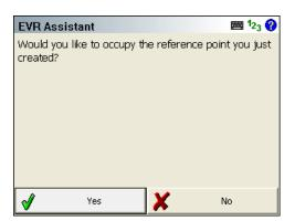
Set the Occupy Point to 1 and set the Instrument Height to 5.5'. At a scene, be sure to measure your Instrument Height and enter that measured height here.
