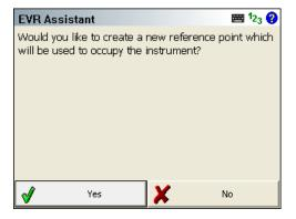
We will begin by assigning an assumed coordinate to the reference point. Create point number 1 at 100,100,100 with a description RP. Then press the **Store Point** button.
