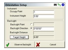
The measurement mode button "BS (Ang/Dist)" indicates that we will be taking an Angle and Distance shot to the backsight.
