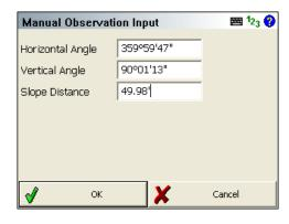
Ensure that your Backsight Error and Distance Error are within your desired tolerances.
