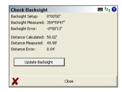
The Check Backsight results are always recorded into the RAW file, so they are there for later scrutiny if necessary.
